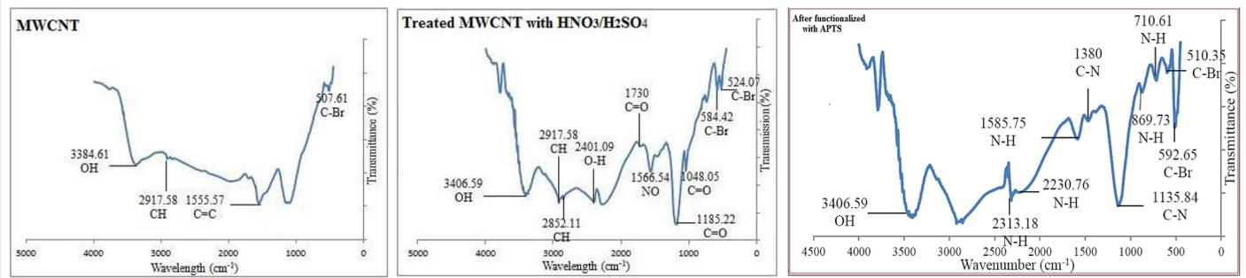
FTIR spectra of treated and untreated MWCNTs
