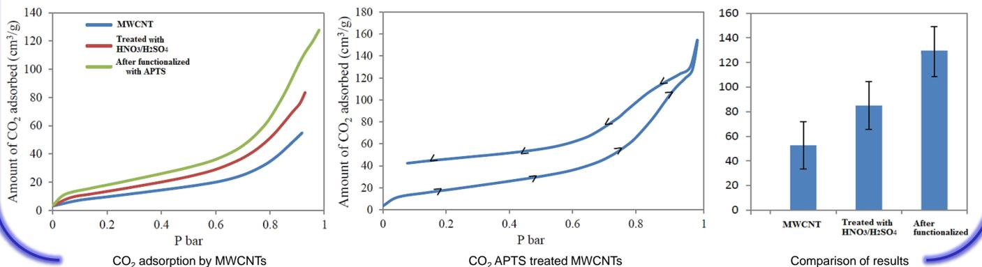
CO<sub>2</sub> adsorption by MWCNTs
