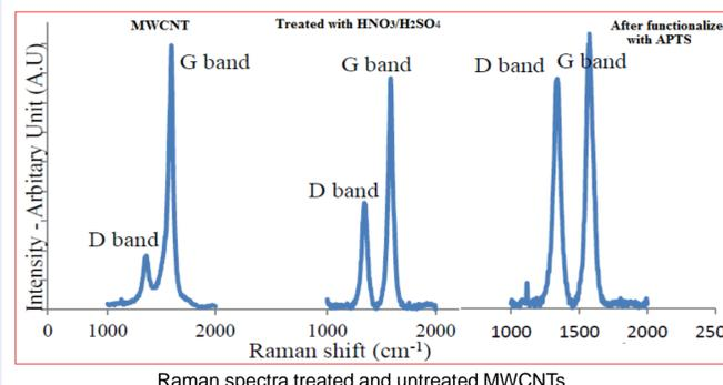
Raman spectra treated and untreated MWCNTs
